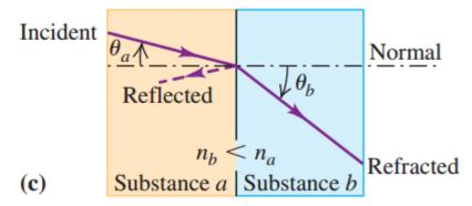
Total internal reflection occurs only if  $n_b < n_a$ .  $\theta_b = 90^{\circ}$   $n_a$   $\theta_{\text{crit}} > \theta_{\text{crit}}$ At the critical angle of incidence,  $\theta_{\text{crit}}$ , the angle of refraction,  $\theta_b = 90^{\circ}$ .
