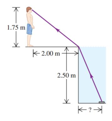
**23.42. Set Up:** The figure below shows a light ray from your cell phone, P, which grazes the corner of the pool, C, and reaches your eyes, E. We assume that the pool is full so that the light exits the water at point C.
