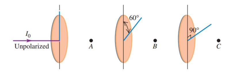
\*23.59. Set Up: When unpolarized light passes through a polarizer the intensity is reduced by a factor of  $\frac{1}{2}$  and the transmitted light is polarized along the axis of the polarizer. When polarized light of intensity  $I_{\text{max}}$  is incident on a polarizer, the transmitted intensity is  $I = I_{\text{max}} \cos^2 \phi$ , where  $\phi$  is the angle between the polarization direction of the incident light and the axis of the filter.
